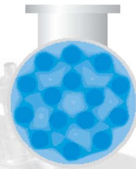
High flow rate and/or poor water quality automatically increase UV radiation intensity
