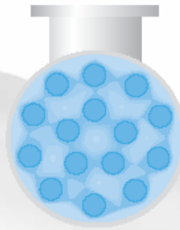
Low flow rate and/or improved water quality automatically reduce UV radiation intensity
